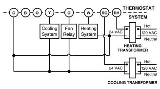
Figure 5. Typical wiring diagram for heat/cool, 5-wire, two-transformer systems with common connection (required)
